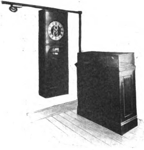
The master clock in the time service department. It operates ninety circuits in New York City on which there are as many as 3,000 synchronized clocks
