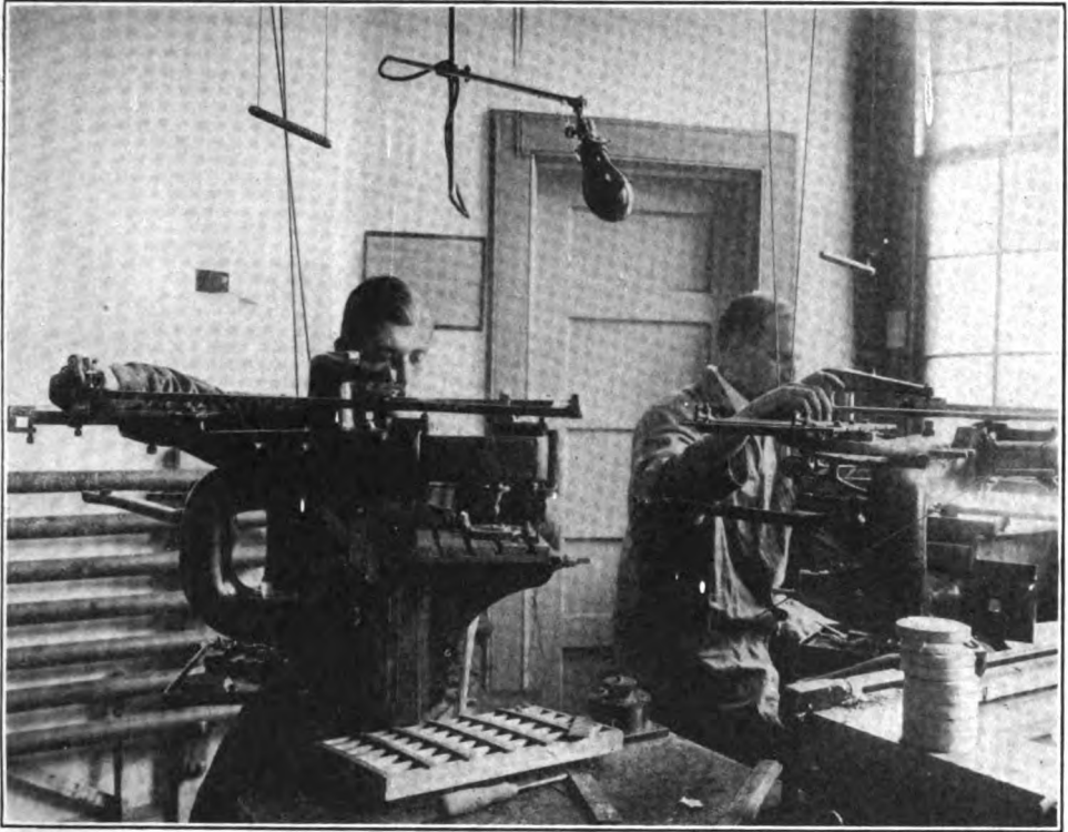
Many of the instruments require special markings, figures, letters and scales. Such work is done in the engraving department, on special machines of the pantograph type.
