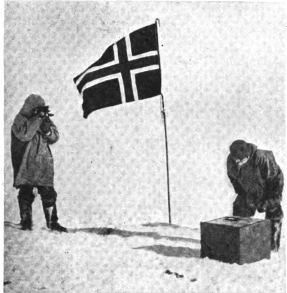
In the photograph Captain Amundsen is seen taking an observation of the sun through a sextant, while one of his assistants examines the "artificial horizon." The flag is planted at the point determined upon as the exact location of the South Pole.
